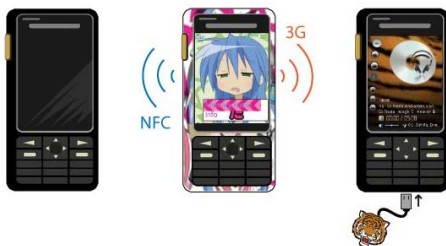
Figure 1. Middle: NFC detects whether tagged shell is near, identifies it and sends the id to a server, which returns software to handheld. Right: Charm is attached to the USB-slot, and software is loaded directly from it.
