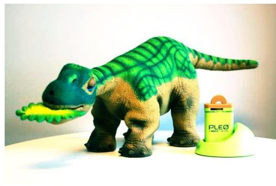
Figure 1. Pleo with leaf and battery in recharger.
