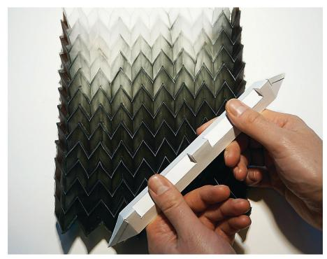
Figure 4. Sketch of the Force tool used for programming a shape-changing material.
