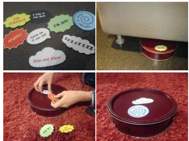
Figure 6. Interaction scenario for simplistic higher level behaviours. By attaching simplistic labels indicating a higher level state of activity, users would be able to put the device into different modes.
