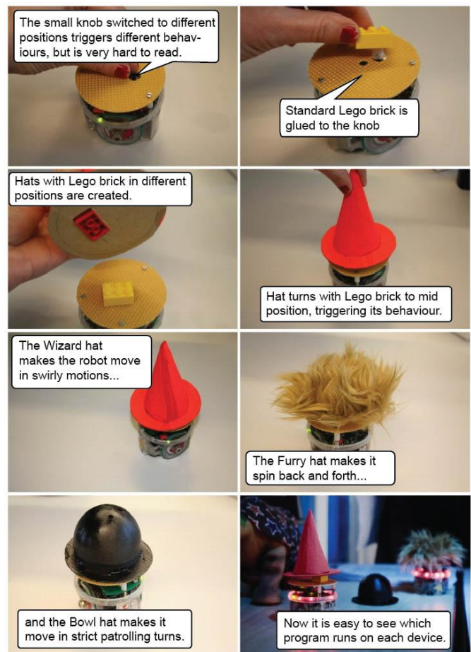
Figure 8. The Hat Trick. A demo illustrating how the changing of hats could simplify control and provide a clearer view of the position of a small knob that triggers different movement patterns of a device.
