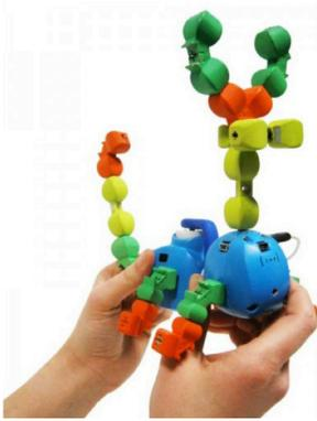
Figure 4 Programming by example: Topobo being programmed [7].
