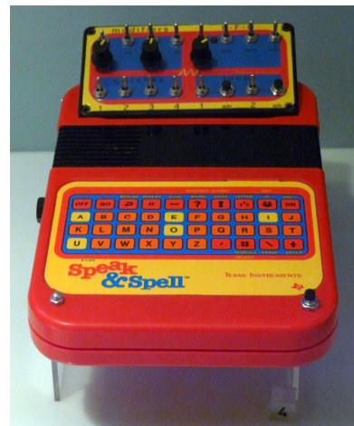
Figure 3 – A Circuit-Bent Speak & Spell, as exhibited at the London Science Museum. Switches, buttons and potentiometers have been added to the device, controlling the modifications made to its circuits (Image copyright Loz Pycok, CC BY-SA).
