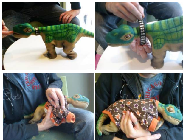
Figure 1. Controlling Pleo using actDresses. From top-left: Playing with the robot in “watchdog” mode, as indicated by bracelet. When user changes the costume from bracelet to pyjama, the robot is slowly switching into sleep mode.
