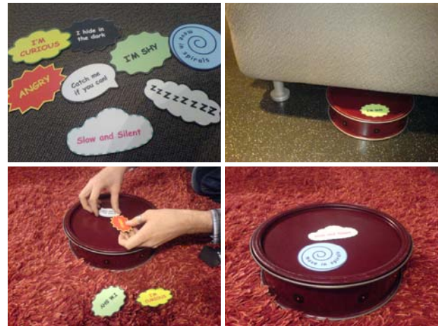
Figure 3. The vacuum robot scenario. A set of signs that can put the robot into different modes. The “shy” sign has made the robot hide under the sofa, and is switched to another mode by the user, to make is spiral slowly and silently on the carpet.
