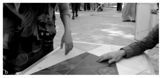
Fig 1. Leather used as a surface material for the touch-sensitive input surface of the *sound box*. The sensory experience of touching leather invited for gestures of gently touching and stroking, which played a significant role in how the touch-sensitive input surface was approached and interacted with.
