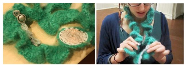
Fig 2. The use of textile and soft materials guided the way the *Speaker Scarf* has been designed, in particular the specific physical manipulations that need to be performed in order to listen to the music. Left: the textile speaker unit and the on/off switch that can be also used for adjusting the volume. Right: Adjusting the volume by placing a metallic button on one of the loops made of resistive yarn.
