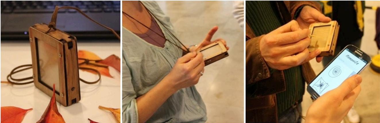
**Figure 1. Memonile Necklace; a) overview picture of the device, b) device in use, c) device next to a smartphone, showing feed tracking the screenless doodles and gestures performed on the Memonile.**
