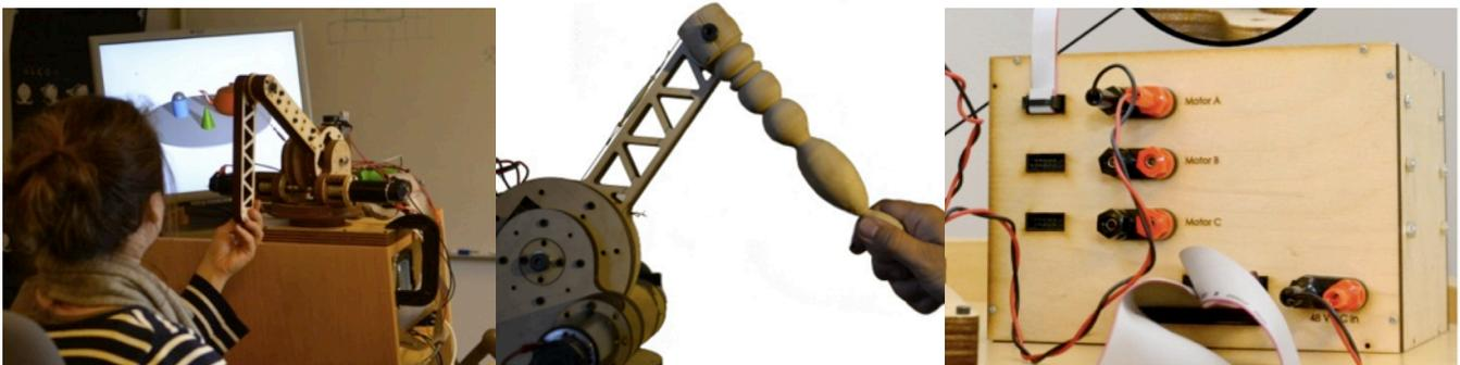
Figure 3. Woody, a haptic feedback device that can be physically adapted to fit the needs of specific haptic manipulation scenarios; a) overview of testing the device with on-screen model, b) the device with another design of arm, c) box with electrical interface.
